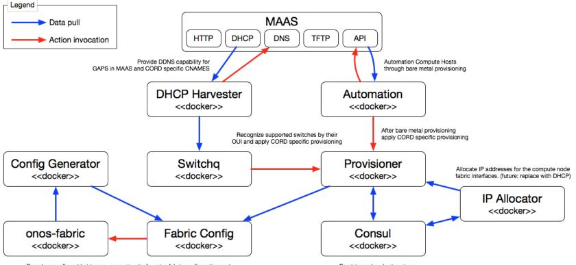
Based on configurable triggers, generate a leaf - spine fabric configuration and update the onos fabric controller (generation available today, automation future) Persistence key / value store
