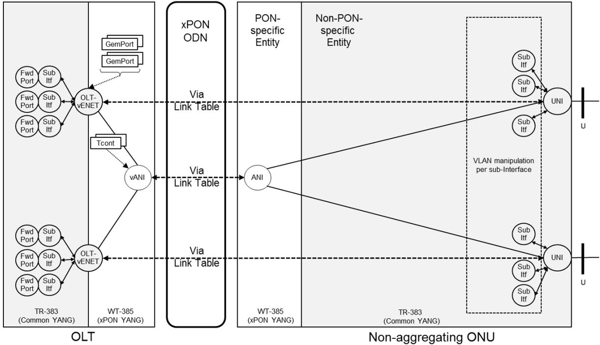
**Figure 8 – Ethernet Service Model Example (Simplified Combined-NE mode with Non-aggregating ONU)**
