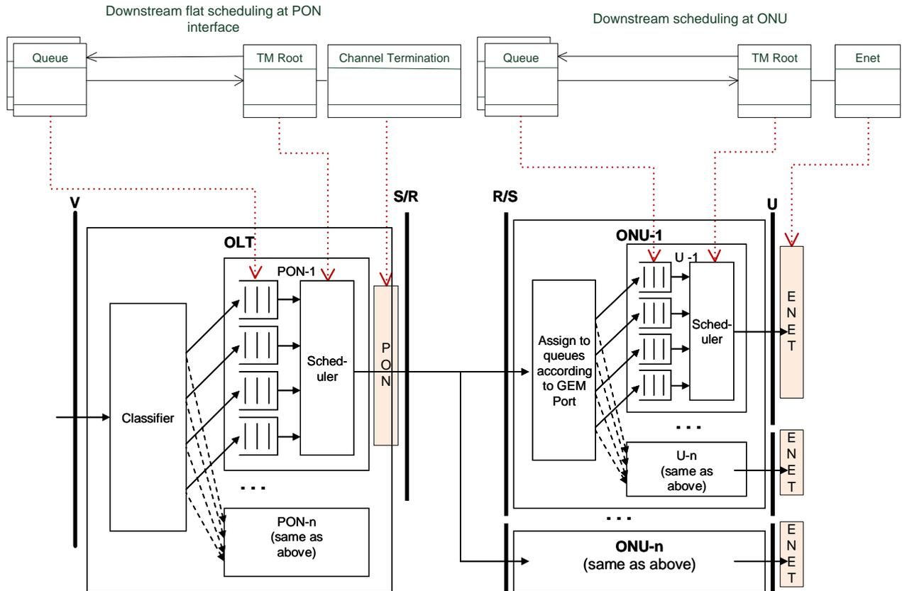
Figure 10 – Downstream Scheduling and Queuing Model Example
