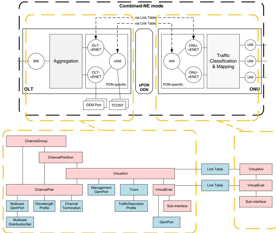
**Figure 5 – Ethernet Service Configuration using xPON YANG and Common YANG**
