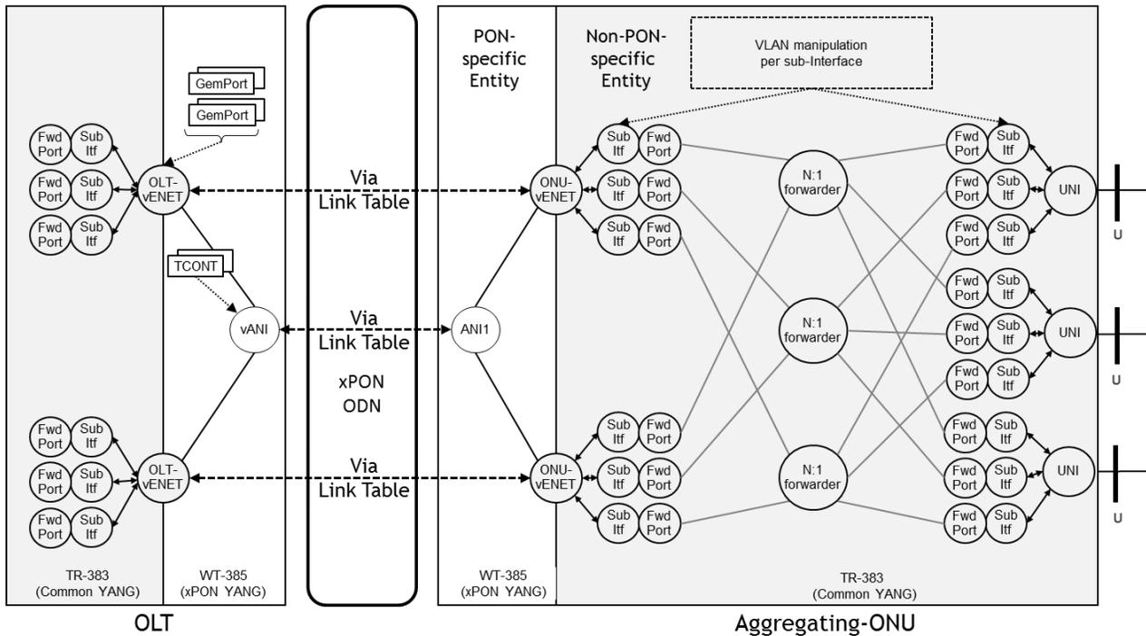
**Figure 6 – Ethernet Service Model (Combined-NE mode with Aggregating ONU)**
