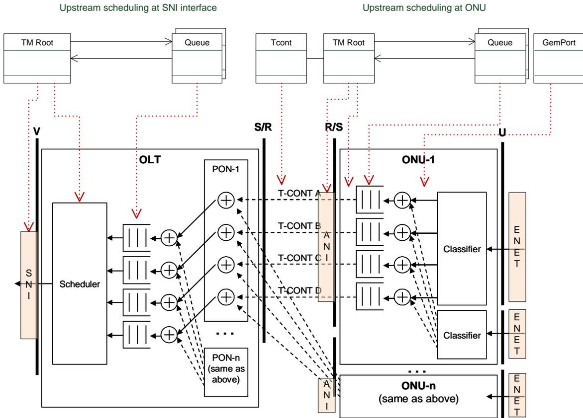
Figure 9 – Upstream Scheduling and Queuing Model Example
