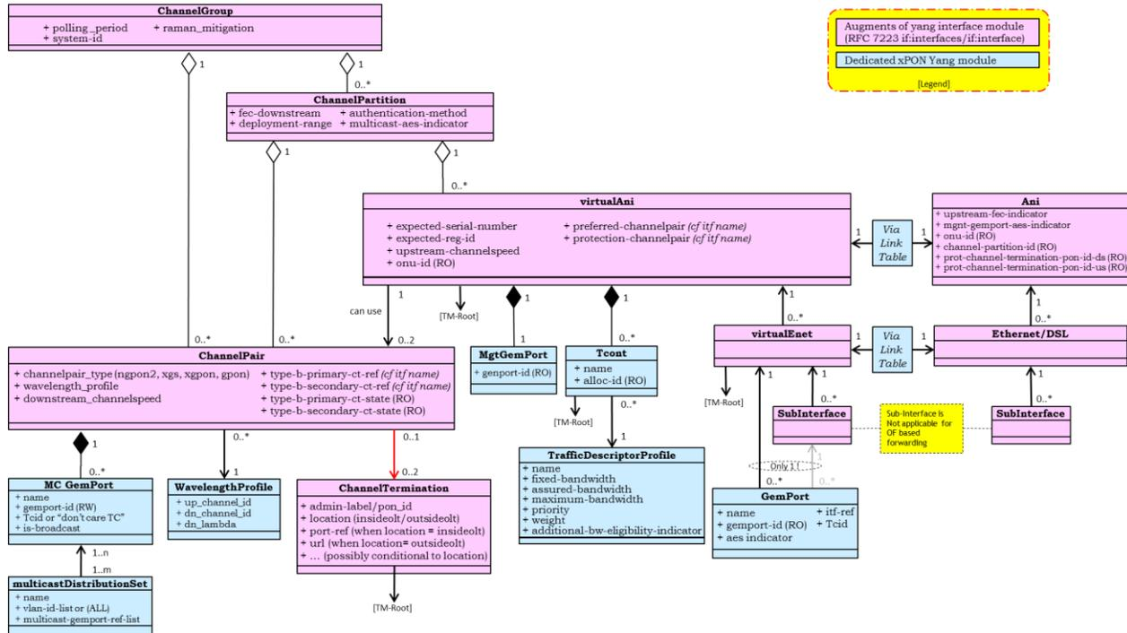
Figure 13 – xPON YANG UML Model
